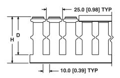
For 75mm and 100mm height duct
