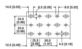
For 75mm and 100mm width duct\*
