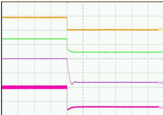
(VIN = 5 V, VOUT = 1.8 V, IOU = 3 A) Upper Trace: Enable Pin Voltage, 5 V / div Second Trace: Power Good Pin Voltage, 5 V / div Third Trace: Output Voltage, 2 V / div Lower Trace: Inductor Current, 2 A / div Time = 200 \mu s / div
