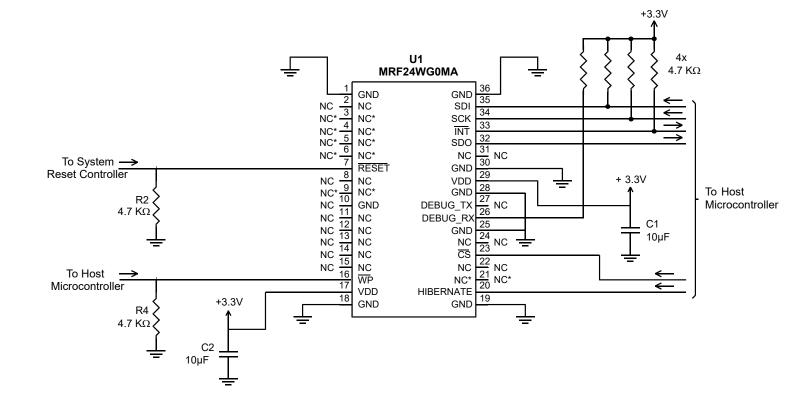
**Note:** The example application schematic is for suggested design purposes. Please refer to Table 1-1 in Section 1.0 "Device Overview" for the module pin descriptions.
