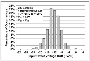
**FIGURE 2-5:** Input Offset Voltage Drift with  $T_A = +25^{\circ}$ C to  $+125^{\circ}$ C and  $V_{DD} = 5.5V$ .
