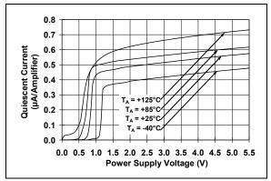
FIGURE 2-21: Quiescent Current vs. Power Supply Voltage.
