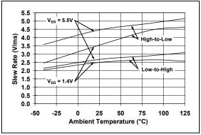
*FIGURE 2-26:* Slew Rate vs. Ambient Temperature.
