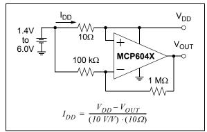
FIGURE 4-7: High-Side Battery Current Sensor.
