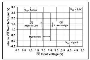
**FIGURE 2-35:** Chip Select  $(\overline{CS})$  Hysteresis (MCP6043 only).
