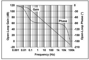
FIGURE 2-14: Open-Loop Gain, Phase vs. Frequency.
