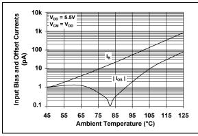
**FIGURE 2-13:** Input Bias, Offset Currents vs. Ambient Temperature.
