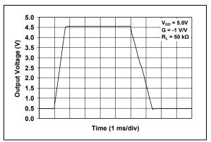
FIGURE 2-34: Large Signal Inverting Pulse Response.
