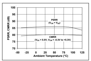
*FIGURE 2-12:* CMRR, PSRR vs. Ambient Temperature.
