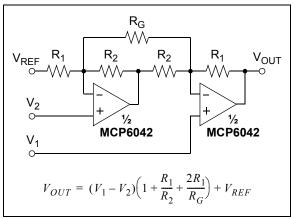
FIGURE 4-8: Two Op Amp Instrumentation Amplifier.
