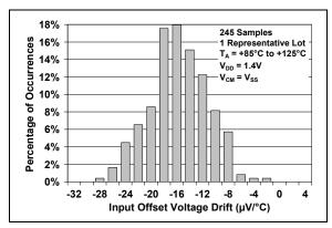
**FIGURE 2-4:** Input Offset Voltage Drift with  $T_A = +85^{\circ}$ C to  $+125^{\circ}$ C and  $V_{DD} = 1.4V$ .
