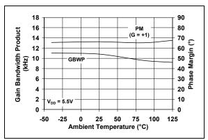
**FIGURE 2-23:** Gain Bandwidth Product, Phase Margin vs. Ambient Temperature with  $V_{DD} = 5.5V$ .
