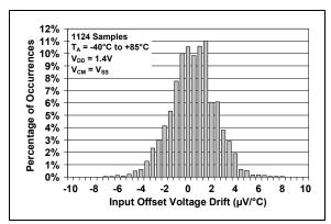
**FIGURE 2-2:** Input Offset Voltage Drift with  $T_A = -40^{\circ}$ C to  $+85^{\circ}$ C.
