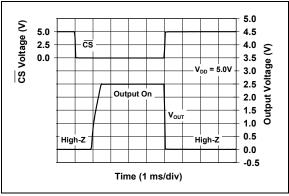
**FIGURE 2-32:** Chip Select ( $\overline{CS}$ ) to Amplifier Output Response Time (MCP6043 only).
