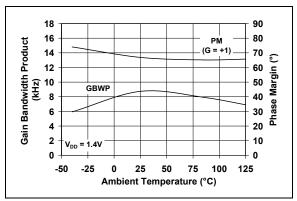
**FIGURE 2-20:** Gain Bandwidth Product, Phase Margin vs. Ambient Temperature with  $V_{DD} = 1.4V$ .
