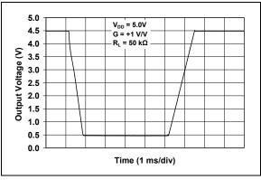
*FIGURE 2-31:* Large Signal Non-inverting Pulse Response.
