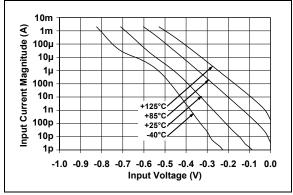
**FIGURE 2-33:** Input Current vs. Input Voltage (below V<sub>SS</sub>).
