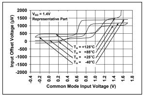
**FIGURE 2-3:** Input Offset Voltage vs. Common-mode Input Voltage with  $V_{DD} = 1.4V$ .
