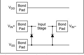
FIGURE 4-1: Simplified Analog Input ESD Structures.
