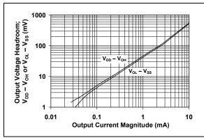
FIGURE 2-25: Output Voltage Headroom vs. Output Current Magnitude.
