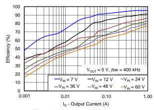
Figure 4. Light-Load Efficiency
