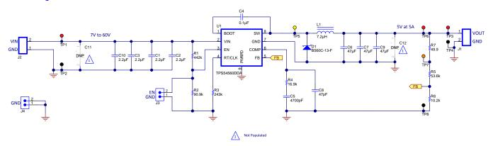
Figure 2. TPS54560EVM-515 Schematic
