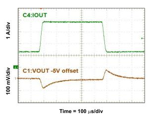
Figure 7. Load Transient Response
