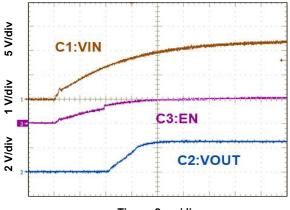
$\label{eq:Time of Time of Time of Time of Time} Time = 2 \text{ ms/div}$  Figure 15. Start Up With  $V_{IN}$  Ramping Up
