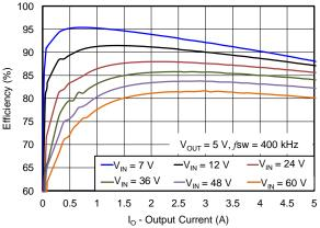
Figure 3. Efficiency Versus Load Current
