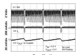
Time = 20  $\mu$ s/div Figure 20. Low Dropout Operation
