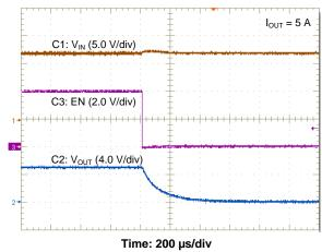
Figure 18. Shutdown With V<sub>IN</sub> Ramping Down
