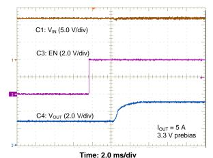
Figure 17. Prebias Start Up With EN Pulled High
