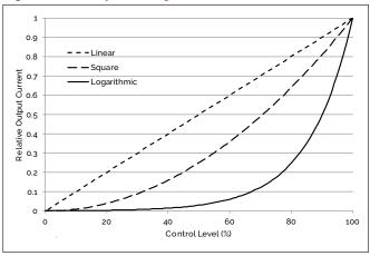
Figure 6: CCT Tuning Characteristics
