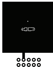
a) 80\text{ }^\circ\text{C}/\text{W} when mounted on a 1\text{ in}^2 pad of 2 oz copper
