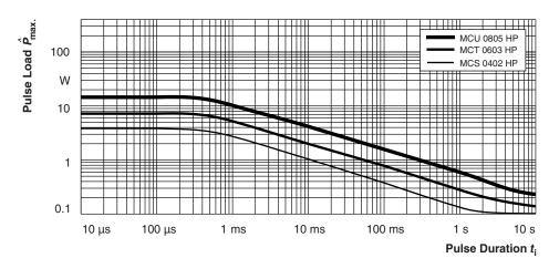
Maximum pulse load, single pulse; applicable if  $\overline{P} \to 0$  and  $n \le 1000$  and  $\hat{U} \le \hat{U}_{max}$ ; for permissible resistance change  $\pm (0.5 \% R + 0.05 \Omega)$
