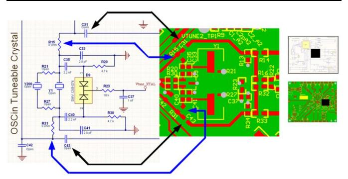
3. Connect charge pump output from PLL1 to Crystal Loop Filter (B1) and Crystal
