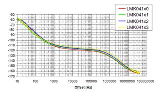
Figure 13. LMK041xx PLL2 Phase Noise (Fout)
