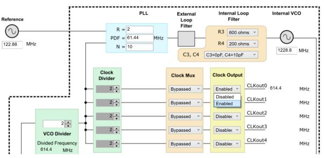
Figure 5. Setting Divider, CLKout\_TYPE, Enabled for CLKoutX on "Bank A" Page
