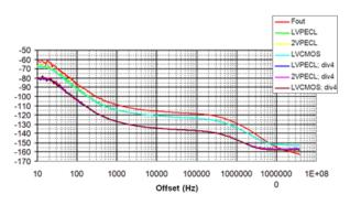
Figure 16. LMK041x2 Phase Noise
