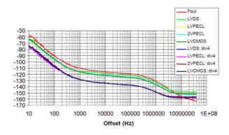
Figure 15. LMK041x1 Phase Noise
