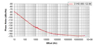
Figure 12. CVHD-950-122.88-MHz VCXO Phase Noise at 122.88 MHz
