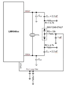
Figure 21. Crystal Oscillator Circuit Diagram
