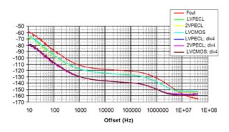
Figure 14. LMK041x0B Phase Noise
