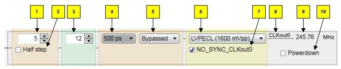
Figure 6. Setting Digital Delay, Clock Divider, Analog Delay and Output Format
