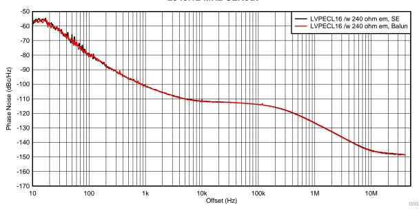
Figure 20. LMK04208, 2949.12 MHz, Divide-by-1
