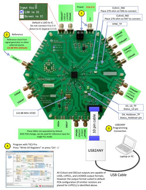
Figure 1. Quick Start Diagram
