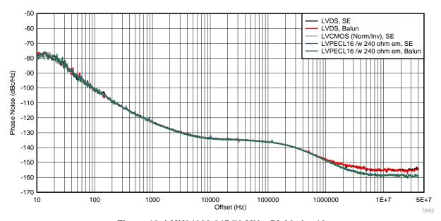
Figure 19. LMK04208 245.76 MHz, Divide-by-12
