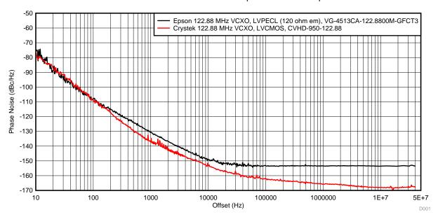
Figure 18. VCXO Phase Noise at 122.88 MHz
