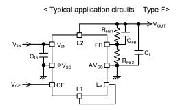
$\label{eq:constraint} \begin{array}{ll} Example of external components (V_{OUT}=1.8V)\\ C_{IN}: 10V/4.7 \mu F (LMK107BJ475KA & TAIYO YUDEN)\\ C_L: 10V/10 \mu F (LMK107BBJ106MA & TAIYO YUDEN)\\ R_{FB1}: 300 k\Omega\\ R_{FB2}: 240 k\Omega\\ C_{FB}: 150 p F (C1005 CH1H151J \ TDK) \end{array}$
