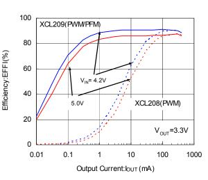
•Efficiency vs. Output Current XCL208x333DR/XCL209x333D
