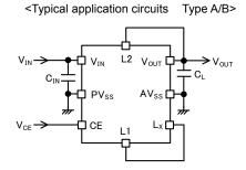
$$\label{eq:components} \begin{split} & \text{Example of external components} \\ & \text{C}_{\text{IN}} : 10\text{V}/4.7\mu\text{F} (\text{LMK107BJ475KA} \quad \text{TAIYO YUDEN}) \\ & \text{C}_{\text{L}} : 10\text{V}/10\mu\text{F} (\text{LMK107BBJ106MA} \quad \text{TAIYO YUDEN}) \end{split}$$
