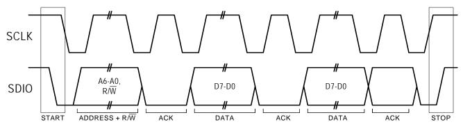
Figure 3. 2-Wire Control Interface Read and Write Timing Diagram
