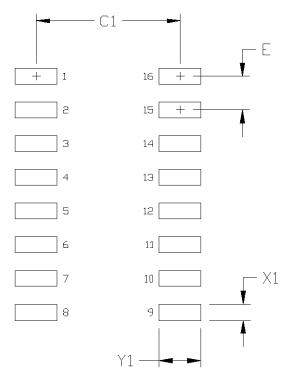
Figure 12.1. 16-Pin Narrow Body SOIC PCB Land Pattern
