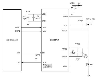
Figure 3.3. Si82395/6/7 Application Diagram
