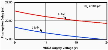
Figure 2.3. Rise/Fall Time vs. Supply Voltage
