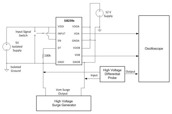
Figure 4.3. CMTI Test Circuit
