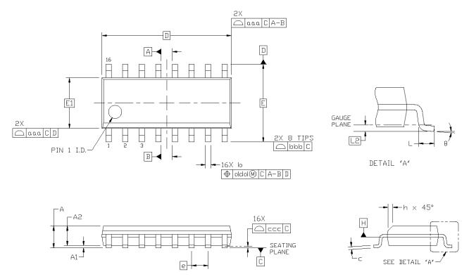
Figure 11.1. 16-Pin Narrow Body SOIC
