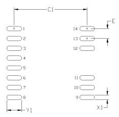
Figure 8.1. 14-Pin WB SOIC Land Pattern
