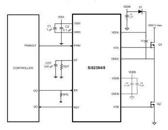
Figure 3.2. Si82394/8 Application Diagram
