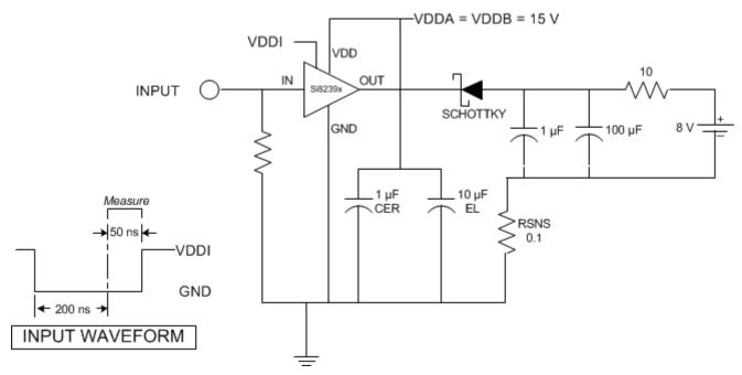
Figure 4.1. IOL Sink Current Test
