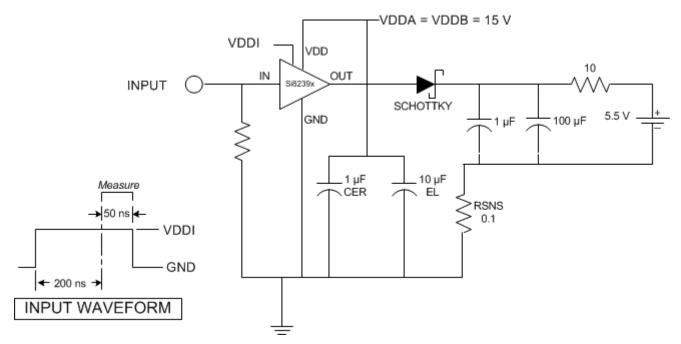
Figure 4.2. IOH Source Current Test
