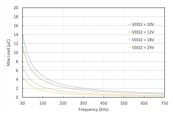
Figure 2.15. Max Load vs. Switching Frequency
