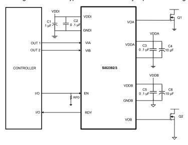
Figure 3.1. Si82392/3 Application Diagram
