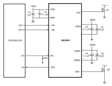
Figure 3.4. Si82390/1 with Enhanced UVLO Feature Application Diagram
