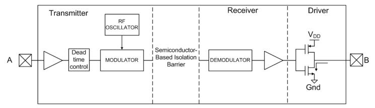
Figure 2.1. Simplified Channel Diagram
