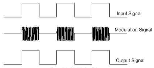
Figure 2.2. Modulation Scheme
