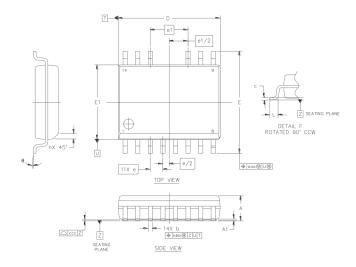
Figure 7.1. Si8239x 14-pin WB SOIC Outline
