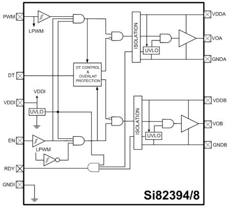
Figure 5.3. Si82394/98 Single-Input High-Side/Low-Side Isolated Drivers
