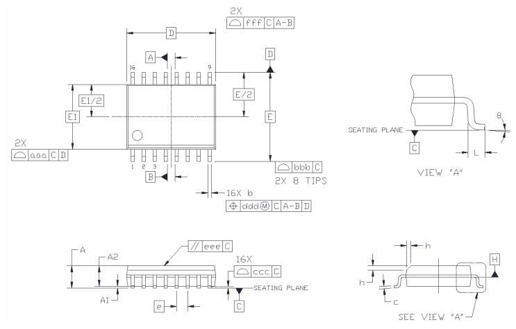
Figure 9.1. 16-Pin Wide Body SOIC
