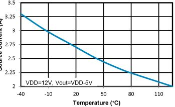
Figure 2.13. Output Sink Current vs. Temperature
