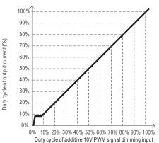
Note: 1. Min. duty cycle of output current is about 9% and the output current is not defined when 0%< Iout<9%.
