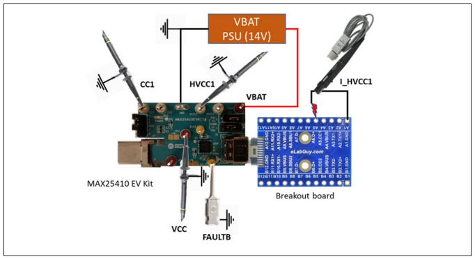
Figure 4. V<sub>CONN</sub> Short-to-Ground Setup
