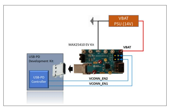
Figure 6. External V<sub>CONN</sub> Control
