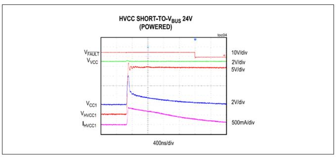
Figure 3. HVCC Short-to-V<sub>BUS</sub> Response
