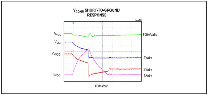
Figure 5. V<sub>CONN</sub> Short-to-Ground Response
