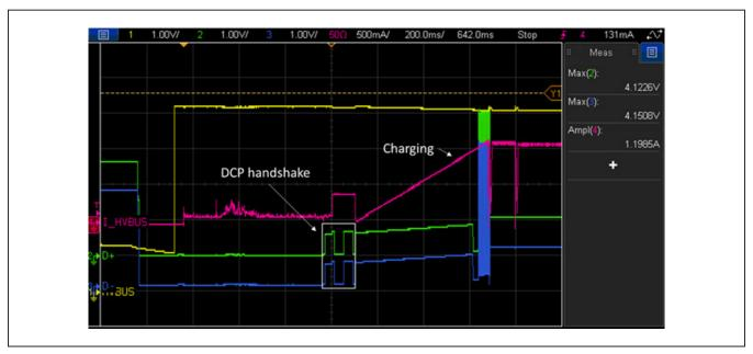
Figure 12. Auto-DCP Response with an Android phone
