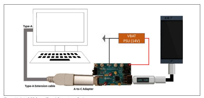
Figure 11. Auto-DCP Setup (Type-A Downstream Port)
