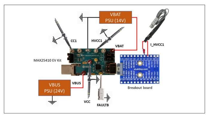
Figure 2. CC Short-to-V<sub>BUS</sub> Setup
