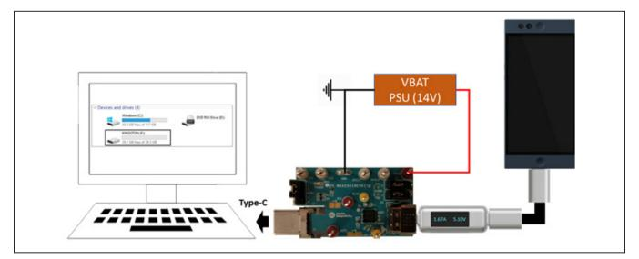
Figure 7. Auto-CDP Setup (Type-C Downstream Port)
