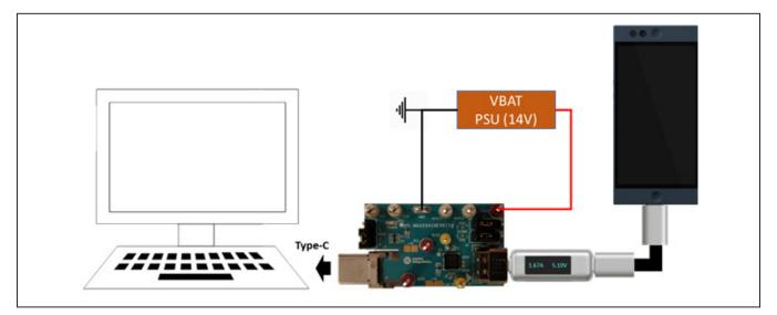
Figure 10. Auto-DCP Setup (Type-C Downstream Port)
