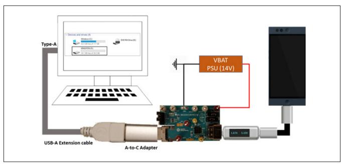
Figure 8. Auto-CDP Setup (Type-A Downstream Port)
