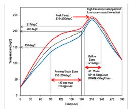
CAUTION: Do not reflow the DC-DC converter as follows, because the DC-DC converter may fall from the substrate during reflowing.
