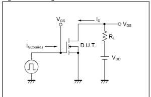
Fig.3-1 Avalanche Measurement Circuit
