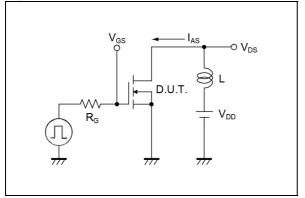
Fig.4-1 trr Measurement Circuit
