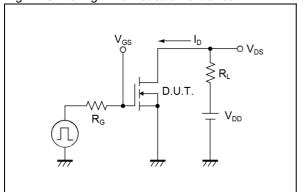
Fig.2-1 Gate Charge Measurement Circuit
