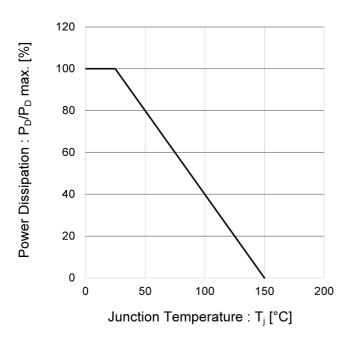
Fig.2 Drain Current Derating Curve
