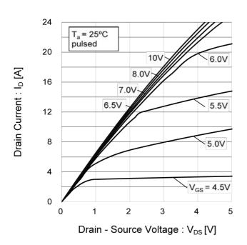
Fig.8 Typical Output Characteristics(II)
