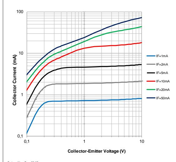
Testcondition:  $T_{\Lambda} = 25 \, ^{\circ}\text{C}$ CHECKED REVISION DATE (YYYY-MM-DD) GENERAL TOLERANCE WE 001.004 2022-01-05 DIN ISO 2768-1m **WL-OCPT Optocoupler** Würth Elektronik eiSos GmbH & Co. KG **Phototransistor** WÜRTH EMC & Inductive Solutions Max-Eyth-Str. 1 140816142400 **ELEKTRONIK** 74638 Waldenburg SIZE/TYPE STATUS Tel. +49 (0) 79 42 945 - 0 BUSINESS UNIT PAGE YOU EXPECT www.we-online.com DIP 4 eiPal Valid 5/12 eiSos@we-online.com
