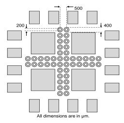
For best result, use a thermal via array as proposed in the picture above with drill of max 200µm, annular ring diameter of 400µm is recommended, vias spaced 500µm apartEnsure enough copper area is used for heat-sinking, to keep the junction temperature below 125°C.
