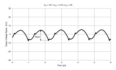
In case the application has more demanding requirements in terms of output voltage ripple, additional external capacitors should be used. The value of the external additional capacitance (C<sub>OUT,INT</sub>) can be calculated using the following equation:
