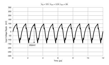
If the application has more demanding requirements in terms of input voltage ripple, an external input capacitor can be placed.
