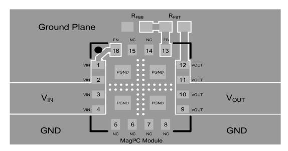
The ground connection of the lower resistor of the output voltage divider (R<sub>FBB</sub>) should be routed to the PGND pins of the device. If not properly handled, poor grounding can result in degraded load regulation or erratic output voltage ripple behaviour.
