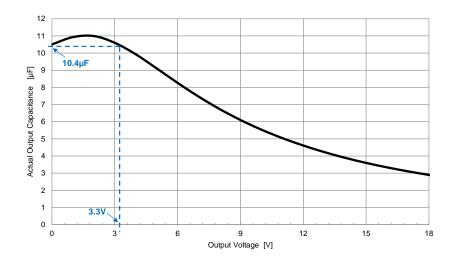
At  $V_{OUT}$  = 3.3V the value of the output capacitance is not reduced due to the voltage, it is instead slightly higher. Nevertheless, a total value of 20µF can be considered for  $C_{OUT, \, INT}$ .
