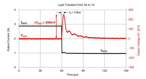
If the application demands a lower undershoot or overshoot, an additional external capacitance is necessary. In order to choose the value of the external output capacitor Cout, Ext, the following steps should be utilized:
