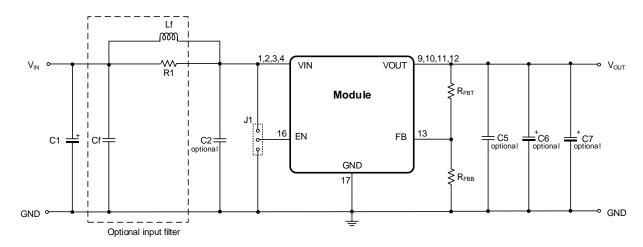
The 171031801 integrates both the input and output capacitors. Therefore, additional external input/output capacitors are normally not required.
