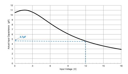
From the diagram above, the actual capacitance value of  $4.7\mu F$  can be read.
