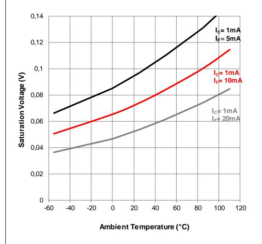
Testcondition:  $I_F$ = 5 mA; Normalized to  $T_{\Delta}$  = 25 °C
