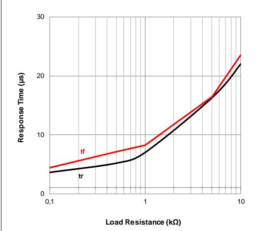
Testcondition:  $I_F = 5$  mA;  $T_{\Delta} = 25$  °C
