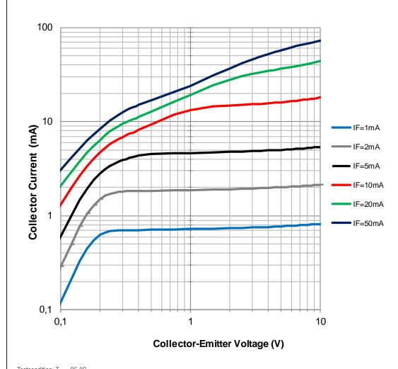
Testcondition:  $T_{\Lambda} = 25 \, ^{\circ}\text{C}$ CHECKED REVISION DATE (YYYY-MM-DD) GENERAL TOLERANCE WE 001.004 2022-01-05 DIN ISO 2768-1m **WL-OCPT Optocoupler** Würth Elektronik eiSos GmbH & Co. KG **Phototransistor** WÜRTH EMC & Inductive Solutions Max-Eyth-Str. 1 140816142000 **ELEKTRONIK** 74638 Waldenburg SIZE/TYPE STATUS Tel. +49 (0) 79 42 945 - 0 BUSINESS UNIT PAGE YOU EXPECT www.we-online.com DIP 4 eiPal Valid 5/12 eiSos@we-online.com
