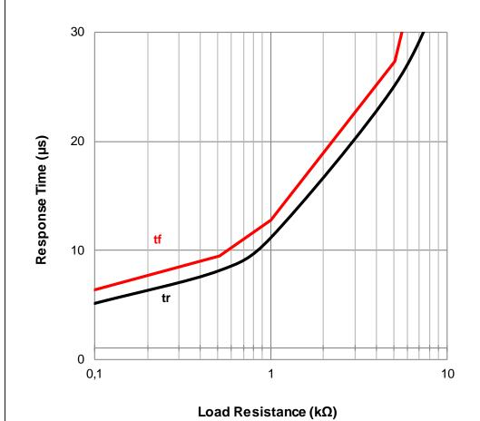
Testcondition:  $I_F = 5mA$ ;  $TA = 25^{\circ}C$ Testcondition:  $I_C = 2mA$ ;  $V_{CF} = 2V$ ;  $TA = 25^{\circ}C$
