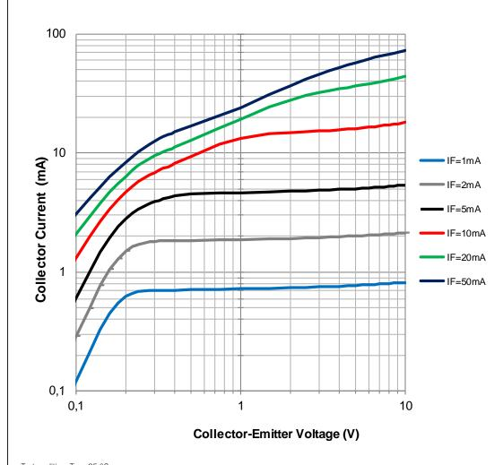
Testcondition:  $T_{\Lambda} = 25 \, ^{\circ}\text{C}$ CHECKED REVISION DATE (YYYY-MM-DD) GENERAL TOLERANCE WE 001.004 2022-01-05 DIN ISO 2768-1m **WL-OCPT Optocoupler** Würth Elektronik eiSos GmbH & Co. KG **Phototransistor** WÜRTH EMC & Inductive Solutions Max-Eyth-Str. 1 140816142300 **ELEKTRONIK** 74638 Waldenburg SIZE/TYPE STATUS Tel. +49 (0) 79 42 945 - 0 BUSINESS UNIT PAGE YOU EXPECT www.we-online.com DIP 4 eiPal Valid 5/12 eiSos@we-online.com
