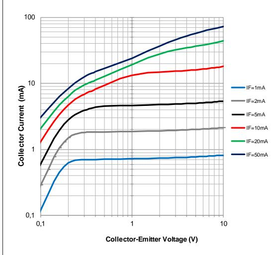
Testcondition:  $T_{\Lambda} = 25 \, ^{\circ}\text{C}$ CHECKED REVISION DATE (YYYY-MM-DD) GENERAL TOLERANCE SaVoq 001.004 2022-01-05 DIN ISO 2768-1m **WL-OCPT Optocoupler** Würth Elektronik eiSos GmbH & Co. KG **Phototransistor** WÜRTH EMC & Inductive Solutions Max-Eyth-Str. 1 140816143000 **ELEKTRONIK** 74638 Waldenburg SIZE/TYPE STATUS Tel. +49 (0) 79 42 945 - 0 BUSINESS UNIT PAGE YOU EXPECT www.we-online.com DIP 4 eiPal Valid 5/12 eiSos@we-online.com
