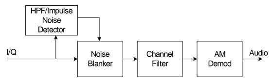
Figure 20. Illustration of Noise Blanker in AM Signal Path.
