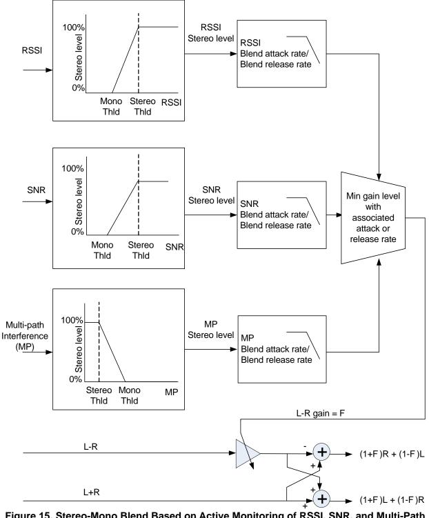
Figure 15. Stereo-Mono Blend Based on Active Monitoring of RSSI, SNR, and Multi-Path Interference
