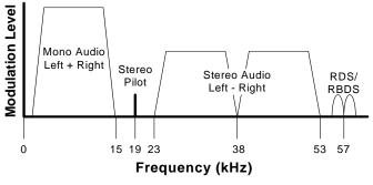
Figure 14. MPX Signal Spectrum
