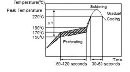
[ Standard Conditions for Reflow Soldering ]
