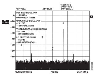
Figure 39. SSB Quadrature Modulator Result Using External 90° Phase Splitter,  $RFP_{IN} = -15 \text{ dBm}$ , VIBB = VQBB = 0.5 V (With Reference to a Common-Mode Voltage of 0.5 V)
