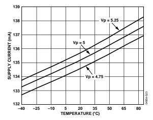
Figure 23. Supply Current vs. Temperature
