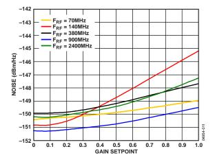
Figure 11. Output Noise Floor vs. Gain Setpoint, No RF Carrier, RF Frequency = 70 MHz, 140 MHz, 380 MHz, 900 MHz, 2400 MHz
