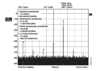
Figure 40. SSB Modulator Applications with Gain and Phase Errors Corrected, RF Pin = -15 dBm, VIBB = VQBB = 0.5 V (With Reference to a Common-Mode Voltage of 0.5 V), I/Q Phase Offset by  $3^{\circ}$ , and Magnitude Offset by 0.5 V
