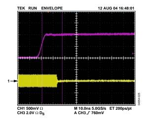
Figure 25. Power Shutdown Response Time, RF = 380 MHz
