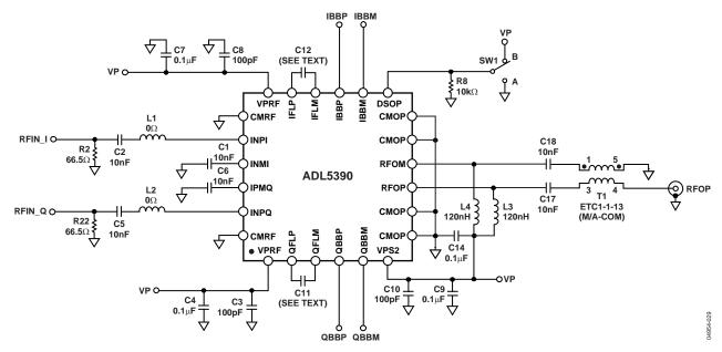
Figure 29. Basic Connections
