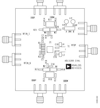
Figure 45. Component Side Layout
