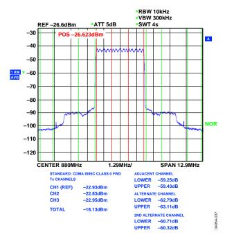
Figure 41. ADL5390 as a Quadrature Modulator with the Use of an External 90°Phase Splitter, RF/LO Power = -1 dBm and Gain Control Inputs Driven Differentially with 0.353  $V_{P-P}$ , 3-Carrier CDMA2000 I/Q Data
