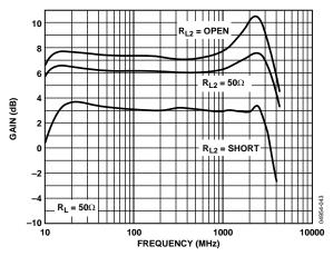
Figure 31. Gain of the ADL5390 Using a Single-Ended Output with Different Dummy Loads,  $R_{L2}$  on the Unused Output, Gain Setpoint = 1.0
