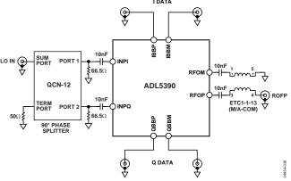
Figure 38. Quadrature Modulator Application
