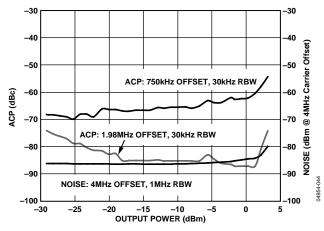
Figure 36. Noise and ACP vs. Output Power, Single-Carrier CDMA2000 Test Model,  $V_1 = V_0 = 0.353$ , ACP Measured in 30 kHz RBW at  $\pm 750$  kHz and  $\pm 1.98$  MHz Carrier Offset, Noise Measured at  $\pm 4$  MHz Carrier Offset
