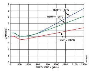
Figure 7. Channel Gain vs. RF Frequency, Temp =  $+85^{\circ}$ C,  $+25^{\circ}$ C,  $-40^{\circ}$ C, Gain Setpoint = 1.0
