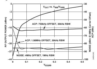
Figure 37. Output Power, Noise, and ACP vs. I and Q Control Voltages, CDMA2000 Test Model,  $V_1 = V_{Q}$ , ACP Measured in 30 kHz RBW at  $\pm 750$  MHz and  $\pm 1.98$  MHz Carrier Offset, Noise Measured at  $\pm 4$  MHz Carrier Offset
