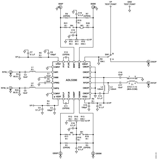
Figure 44. Evaluation Board Schematic
