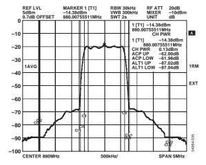
Figure 35. Output Spectrum, Single-Carrier CDMA2000 Test Model at -5 dBm,  $V_1 = V_Q = 0.353$  V, ACP Measured at 750 kHz and 1.98 MHz Carrier Offset, Input Signal–Filtered Using a Cavity-Tuned Filter (Pass Band = 4.6 MHz)
