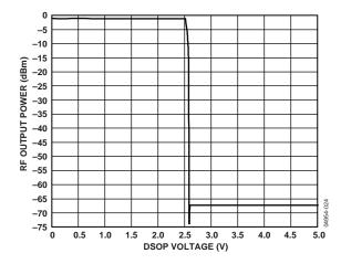
Figure 24. Power Shutdown Attenuation, RF = 380 MHz
