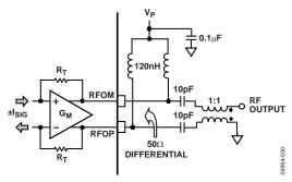
Figure 30. RF Output Interface to the ADL5390 Showing Coupling Capacitors, Pull-Up RF Chokes, and Balun
