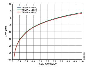
Figure 4. Gain Magnitude vs. Gain Setpoint, Temp =  $+85^{\circ}$ C,  $+25^{\circ}$ C,  $-40^{\circ}$ C, RF Frequency = 380 MHz (Channel I or Channel Q)
