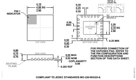
Figure 47. 24-Lead Lead Frame Chip Scale Package [LFCSP] 4 mm × 4 mm Body and 0.75 mm Package Height (CP-24-10) Dimensions shown in millimeters
