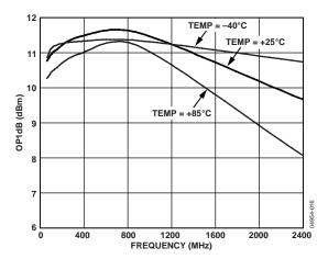
Figure 16. Output 1 dB Compression Point vs. RF Frequency,  $Temp = +85^{\circ}C$ ,  $+25^{\circ}C$ ,  $-40^{\circ}C$ , Gain Setpoint = 1.0
