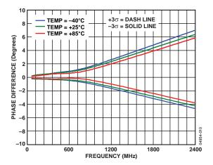
Figure 10. Channel-to-Channel Phase Matching vs. RF Frequency, Temp =  $+85^{\circ}\text{C}$ ,  $+25^{\circ}\text{C}$ ,  $-40^{\circ}\text{C}$ , Gain Setpoint = 1.0
