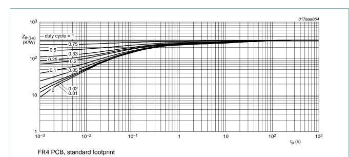
Fig 4. TR2: Transient thermal impedance from junction to ambient as a function of pulse duration; typical values
