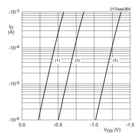
$T_{j} = 25 \, ^{\circ}\text{C}; \, V_{DS} = -5 \, V$
