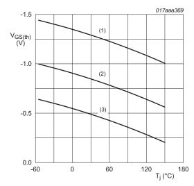
$I_D$  = -0.25 mA;  $V_{DS}$  =  $V_{GS}$
