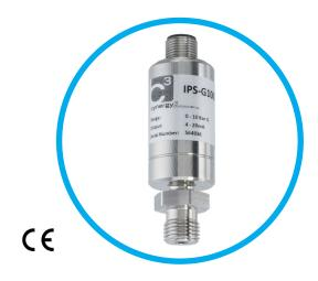
The IPSU-M12 series is suitable for use in a wide range of industrial applications. The probe uses a piezo-resistive ceramic sensor, giving excellent media compatibility within a stainless steel housing.
