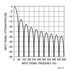
Figure 18. Input Signal Attenuation vs Frequency (Low Frequencies)
