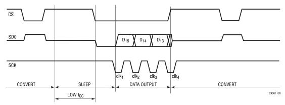
Figure 9. Idle-High (CPOL = 1) Clock and Aborted I/O Example
