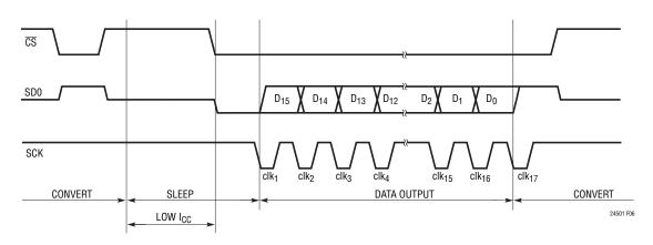
Figure 6. Idle-High (CPOL = 1) Clock Operation Example. A 17th Clock Pulse is Used to Trigger a New Conversion Cycle
