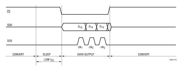
Figure 10. Idle-Low (CPOL = 0) Clock and Aborted I/O Example
