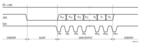
Figure 12. 2-Wire, Idle-High (CPOL = 1) Serial Clock, Operation Example
