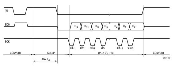
Figure 5. Idle-High (CPOL = 1) Serial Clock Operation Example. The Rising Edge of  $\overline{\text{CS}}$  Starts a New Conversion
