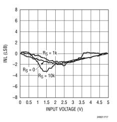
Figure 17. Measured INL vs  $V_{\text{IN}},\,C_{\text{IN}}$  = 0,  $V_{\text{CC}}$  = 5V,  $T_{\text{A}}$  = 25°C
