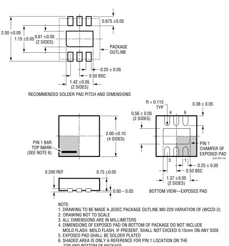
DC Package 6-Lead Plastic DFN (2mm × 2mm) (Reference LTC DWG # 05-08-1703)
