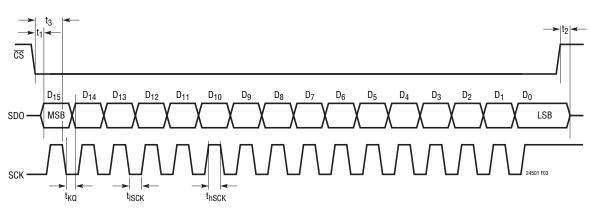
Figure 3. Data Output Timing
