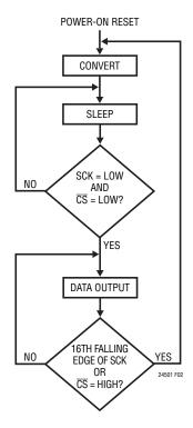
Figure 2. LTC2450-1 State Transition Diagram
