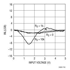
Figure 16. Measured INL vs Input Voltage,  $C_{IN}$  = 0.1µF,  $V_{CC}$  = 5V,  $T_A$  = 25°C
