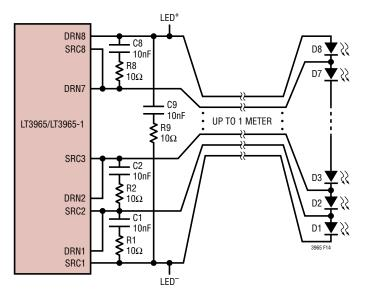
Figure 14. RC Snubbers In Long Wire Application
