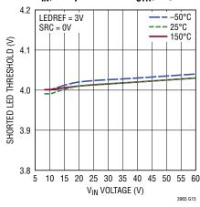
Shorted LED Threshold Falling vs  $V_{IN}$ , Temperature for  $V_{STH}[1:0] = 10$
