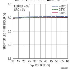
Shorted LED Threshold Falling vs  $V_{IN}$ , Temperature for  $V_{STH}[1:0] = 11$
