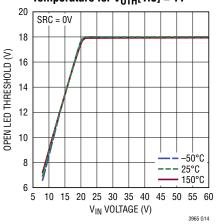
Shorted LED Threshold Falling vs  $V_{IN}$ , Temperature for  $V_{OTH}[1:0] = 00$
