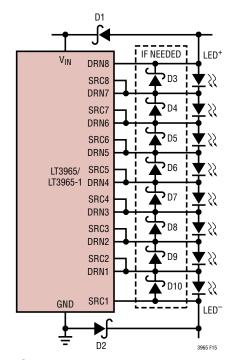
Figure 15. Clamping Diode For LT3965/LT3965-1 Protection
