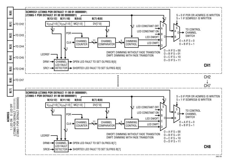
Figure 5. LT3965/LT3965-1 Command Registers and Channel Control Diagram
