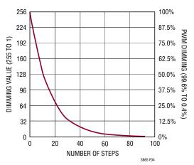
Figure 4. LT3965/LT3965-1 Down Transition Dimming Curve
