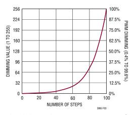
Figure 3. LT3965/LT3965-1 Up Transition Dimming Curve
