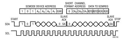
Figure 8. LT3965/LT3965-1 I<sup>2</sup>C Serial Port SCMODE Write Short Format Protocol
