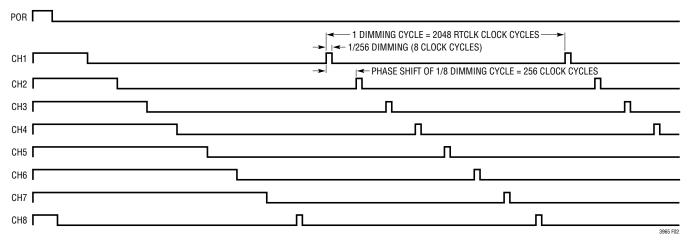
Figure 2. POR Dimming Cycle Initialization Diagram
