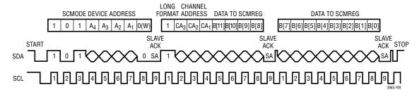
Figure 9. LT3965/LT3965-1 I<sup>2</sup>C Serial Port SCMODE Write Long Format Protocol
