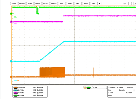
Figure 30. Digit enable startup ( V_{in} = V_{CC} = 24\text{ V} , V_{out} = 0x64\text{ (5 V)} , no load)
