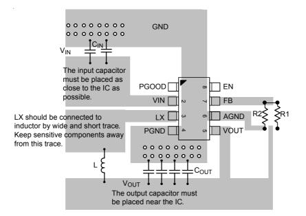
Figure 6. PCB Layout Guide
