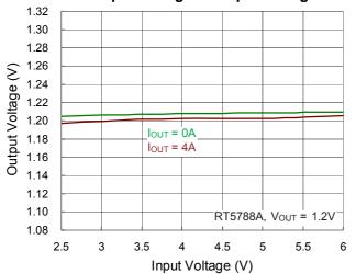
Output Voltage vs. Input Voltage
