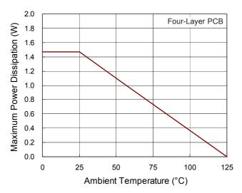
Figure 5. Derating Curve of Maximum Power Dissipation
