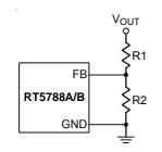
Figure 4. Output Voltage Setting
