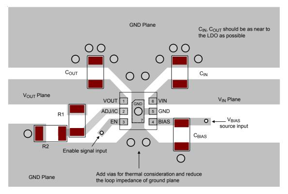
Figure 4. PCB Layout Guide
