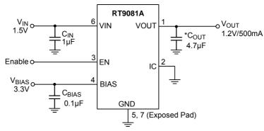
Figure 1. Fixed Voltage Regulator
