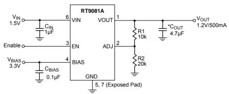
Figure 2. Adjustable Voltage Regulator
