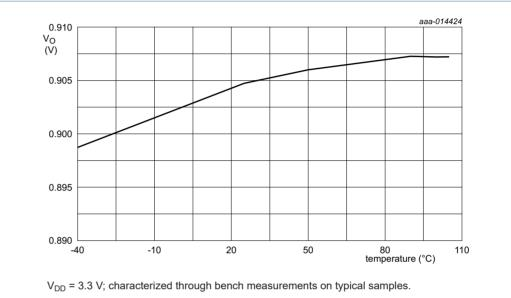
Fig 32. Typical internal voltage reference output voltage
