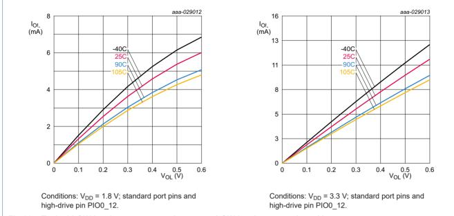
Fig 22. Typical LOW-level output current  $I_{OL}$  versus LOW-level output voltage  $V_{OL}$
