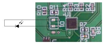
Figure 7. Using a Photodiode with the High-Current Linearity Correction Circuitry
