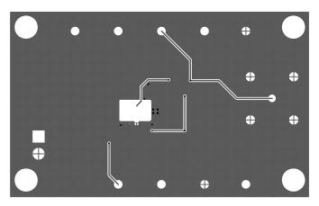
Figure 17. LOG114EVM: Bottom Copper Layer
