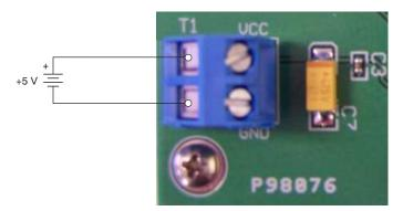
Figure 6. Connecting the 5V Power Supply
