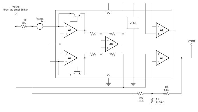
Figure 4. High-Current Linearity Correction Circuit
