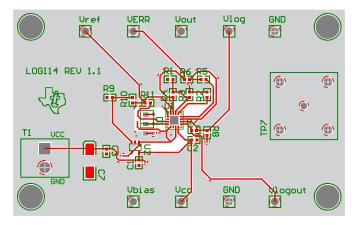
Figure 15. LOG114EVM: Top Side Composite Drawing
