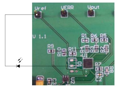
Figure 9. Applying a 0.5-V Reverse Bias to the Photodiode
