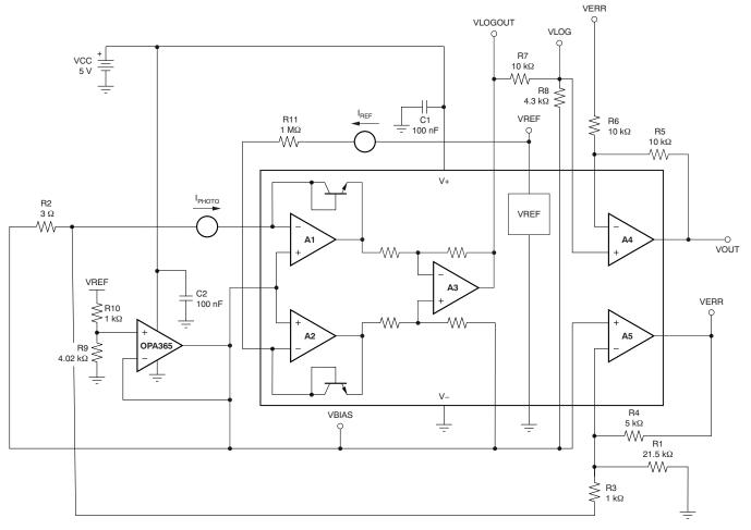
Figure 5. LOG114EVM Complete Circuit
