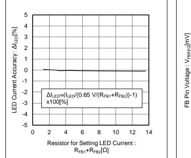
Figure 5. LED Current Accuracy vs Resistor for Setting LED Current
