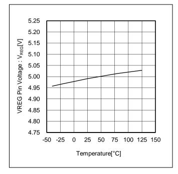
Figure 3. VREG Pin Voltage vs Temperature
