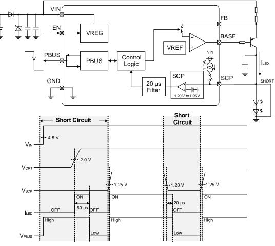
Figure 22. Short Circuit Protection (SCP)
