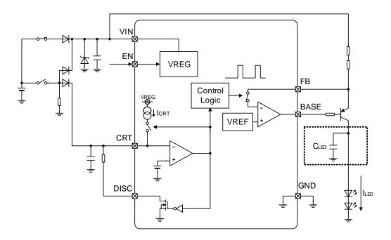
Figure 24. About the Capacitor of Connecting LED Anode
