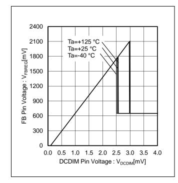
Figure 11. FB Pin Voltage vs DCDIM Pin Voltage
