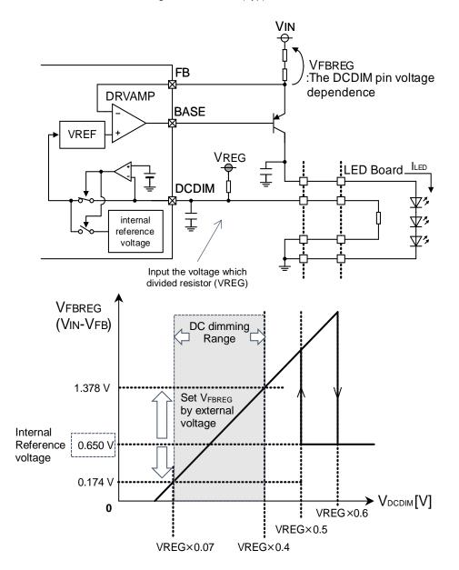
:DC Dimming Gain 730 mV/V(Typ) DDG
