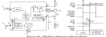
Figure 19. LED Open Detection Timing Chart
