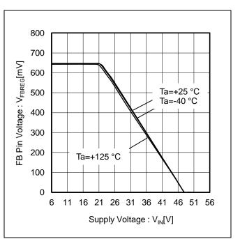
Figure 8. FB Pin Voltage vs Supply Voltage
