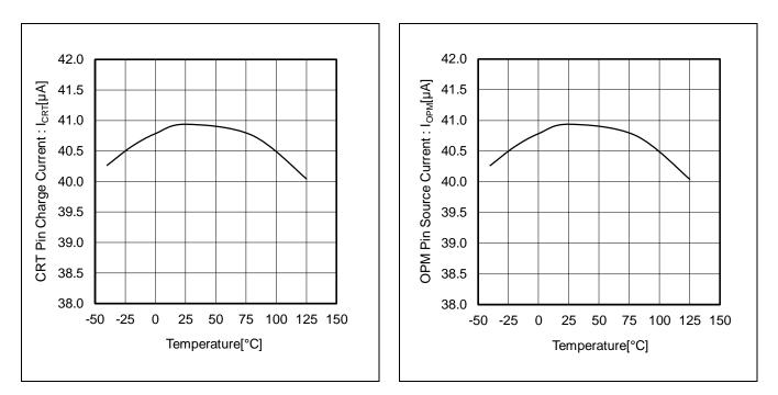
Figure 9. CRT Pin Charge Current vs Temperature
