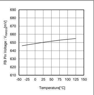
Figure 6. FB Pin Voltage vs Temperature
