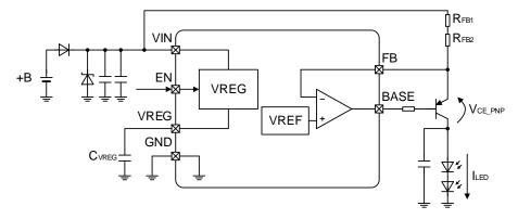
Figure 14. LED Current Setting
