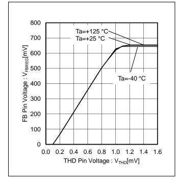
Figure 13. FB Pin Voltage vs THD Pin Voltage
