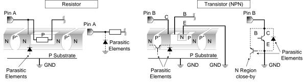
Figure 34. Example of Monolithic IC Structure
