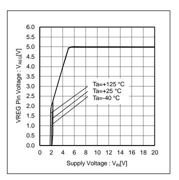
Figure 2. VREG Pin Voltage vs Supply Voltage
