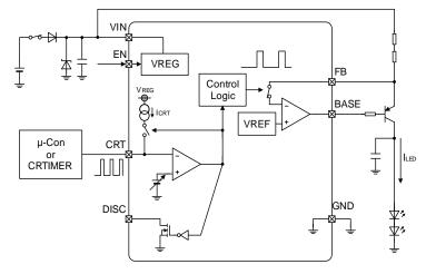
Figure 17. PWM Dimming Operation Using External Signal
