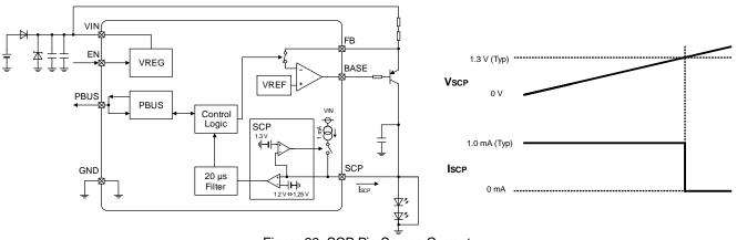
Figure 23. SCP Pin Source Current
