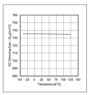
Figure 12. DC Dimming Gain vs Temperature
