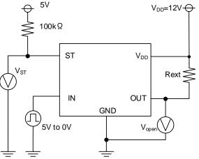
Figure 5. Open Load Detection threshold measuring circuit
