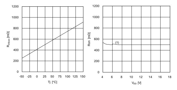
Figure 6. Output ON Resistance Characteristic [temperature characteristic]
