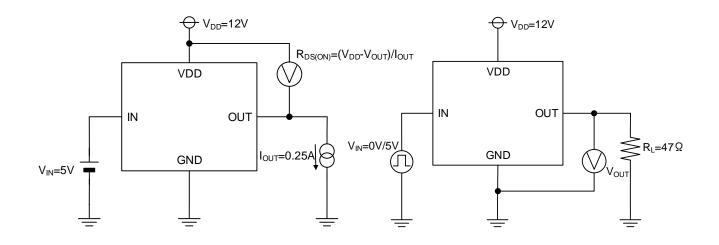
Figure 2. Ron measuring circuit
