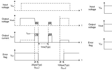
Figure 20. Overcurrent Protect Timing Chart
