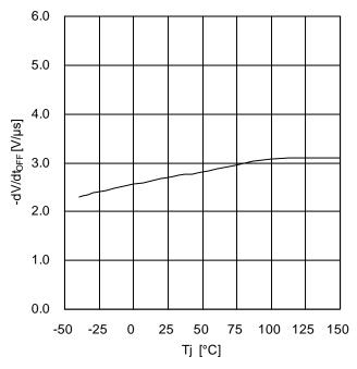
Figure 13. Slew Rate OFF [temperature characteristic]
