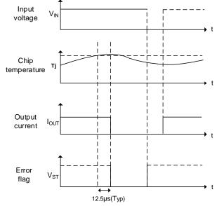
Figure 18. BD1HC500 Off-latch Overheat Protection Timing Chart
