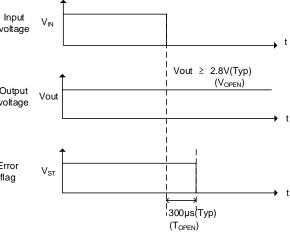
Figure 21. Open Load Detection Timing Chart
