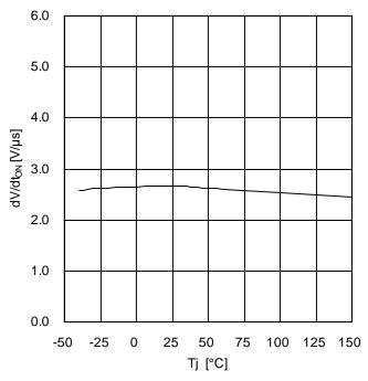
Figure 12. Slew Rate ON [temperature characteristic]
