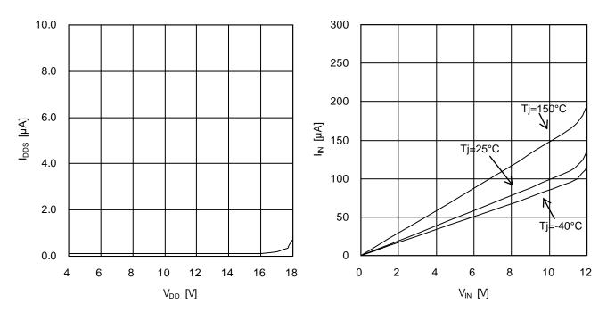
Figure 8. Standby Current Characteristic (V<sub>IN</sub>=0V)
