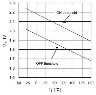
Figure 14. Input Voltage Threshold Characteristic
