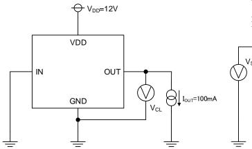
Figure 4. Output clamp voltage measuring circuit
