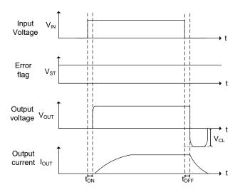
Figure 17. Active Clamp Energy Timing Chart
