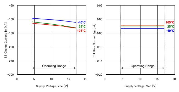
Figure 21. SS Charge Current vs Supply Voltage
