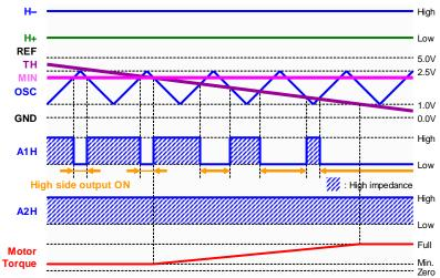
Figure 34. DC input operation timing chart
