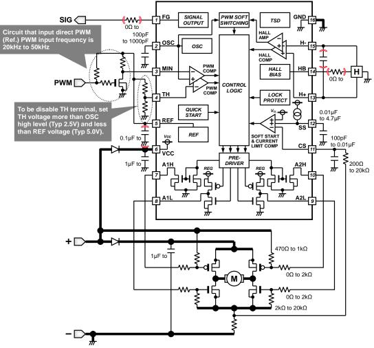
Figure 26. Application of direct PWM input
