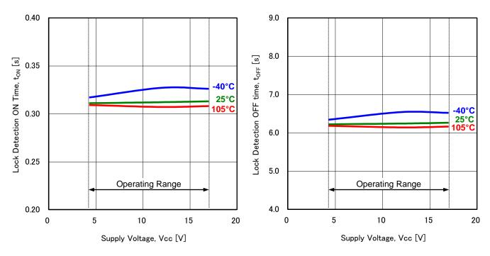
Figure 9. Lock Detection ON Time vs Supply Voltage
