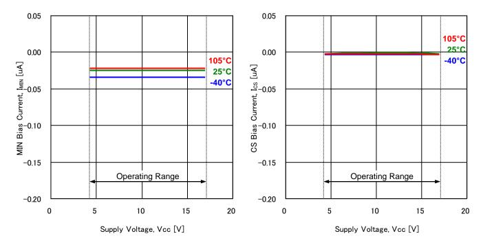
Figure 23. MIN Bias Current vs Supply Voltage
