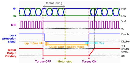
Figure 42. PWM input and quick start timing chart
