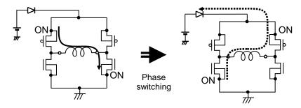
Figure 49. VCC Voltage Rise by Back Electromotive Force
