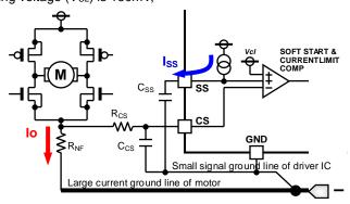
Figure 39. Setting of current limit and ground line
