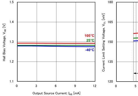
Figure 19. Hall Bias Voltage vs Output Source Current (Vcc=12V)
