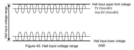
Adjust the value of hall element bias resistor R1 in Figure 44 so that the input voltage of a hall amplifier is input in "Hall Input Voltage" including signal amplitude.
