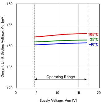
Figure 20. Current Limit Setting Voltage vs Supply Voltage
