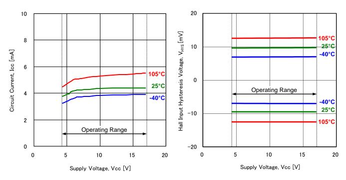
Figure 1. Circuit Current vs Supply Voltage
