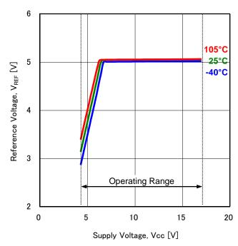
Figure 16. Reference Voltage vs Supply Voltage
