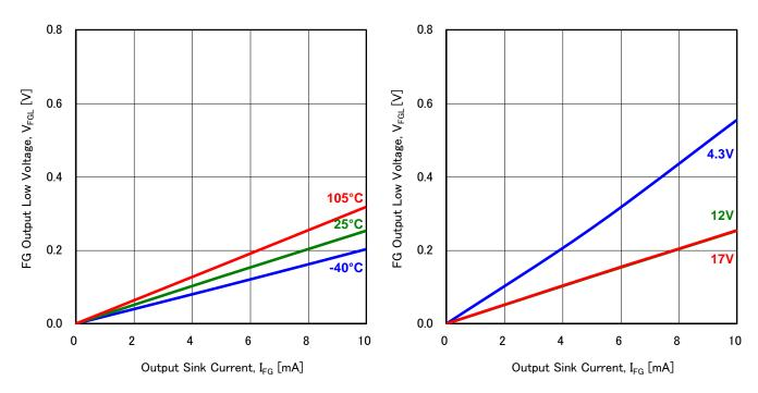
Figure 11. FG Output Low Voltage vs Output Sink Current (Vcc=12V)
