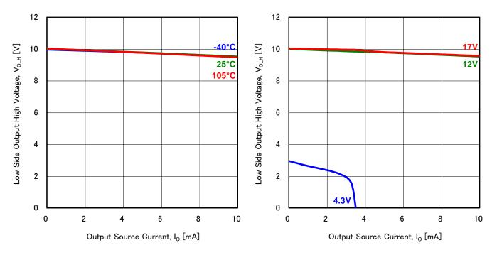
Figure 5. Low Side Output High Voltage vs Output Source Current (Vcc=12V)
