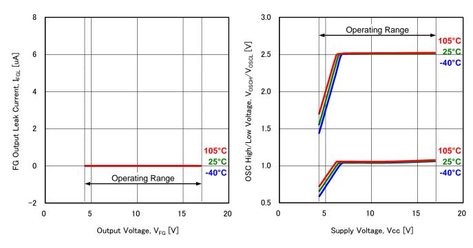
Figure 13. FG Output Leak Current vs Output Voltage
