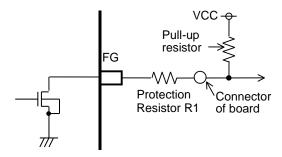
Figure 52. Protection of FG Pin
