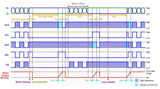
Figure 46. Lock protection (incorporated counter system) timing chart
