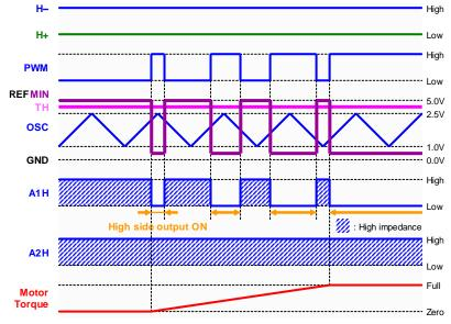
Figure 38. PWM input operation timing chart
