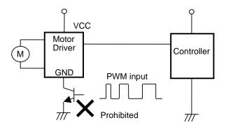
Figure 51. GND Line PWM Switching Prohibited
