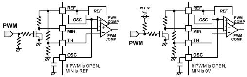
Figure 36. PWM input application 1
