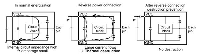
Figure 48. Flow of Current when Power is Connected Reversely
