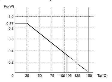
Reduce by 7.0 mW/°C over 25°C. (70.0mm x 70.0mm x 1.6mm glass epoxy board)
