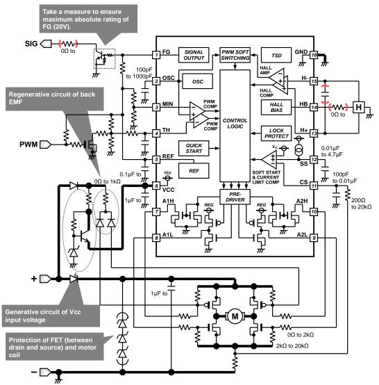
Figure 29. 24V power supply application of PWM input
