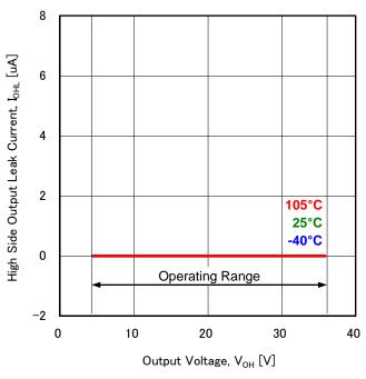
Figure 4. High Side Output Leak Current vs Output Voltage
