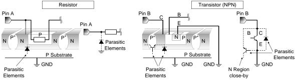
Figure 54. Example of monolithic IC structure
