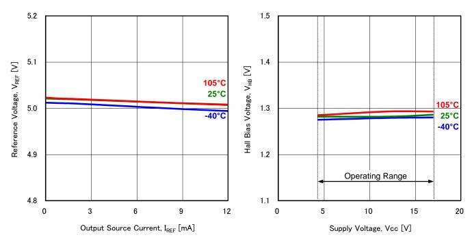
Figure 17. Reference Voltage vs Output Source Current (Vcc=12V)
