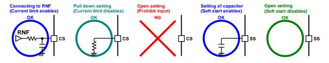
Figure 41. Setting of the current limit and the soft start functions
