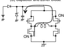
Figure 50. Protection against VCC Voltage Rise
