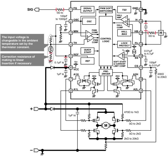
Figure 28. Application of thermistor control
