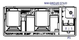
Figure 3. Front View - ACC750-1T24 / ACC750-1T48 Models
