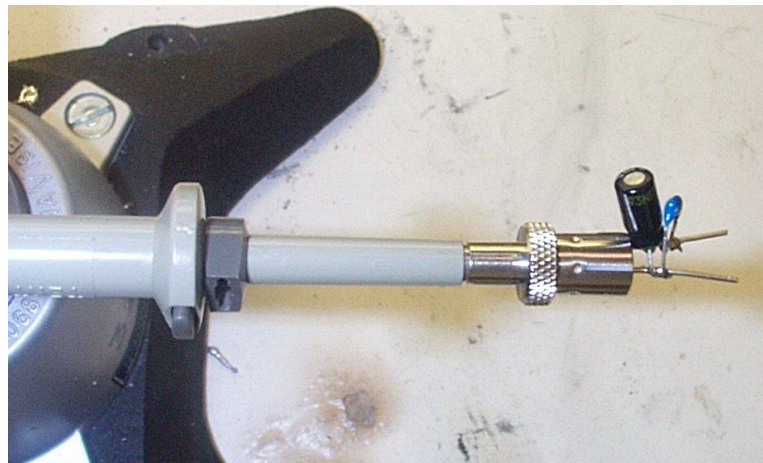
Figure 65 – Oscilloscope Probe with Probe Master ( www.probemaster.com ) 4987A BNC Adapter. (Modified with wires for ripple measurement, and two parallel decoupling capacitors added.)
