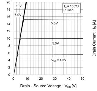
Fig.8 Tj = 150°C Typical Output Characteristics (II)
