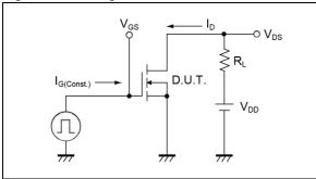
Fig.3-1 Avalanche Measurement Circuit
