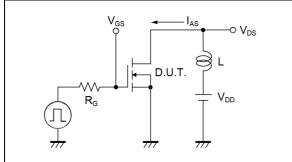
Fig.4-1 dv/dt Measurement Circuit
