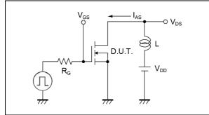
Fig.5-1 di/dt Measurement Circuit
