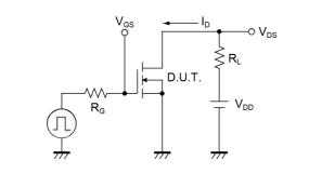
Fig.2-1 Gate Charge Measurement Circuit
