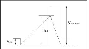
Fig.5-2 di/dt Waveform
