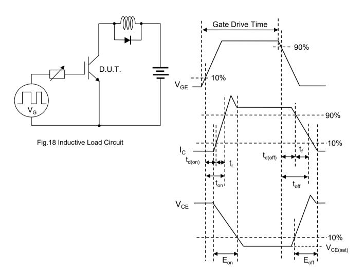
Fig.19 Inductive Load Waveform
