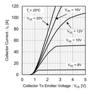
Fig.6 Typical Output Characteristics
