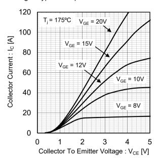
Fig.7 Typical Transfer Characteristics
