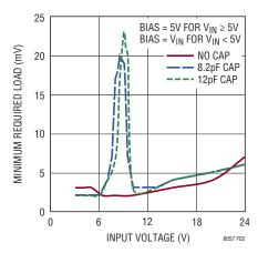
Figure 2. Minimum Required Load vs Input Voltage
