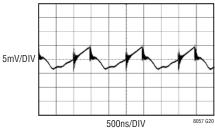
MEASURED ON DC1987 WITH ADDIONAL 1μF AND BNC ATTACHED TO OUTPUT TERMINALS. C7 = 0.1µF. USED HP461A 150MHz AMPLIFIER, SET TO 40dB GAIN.
