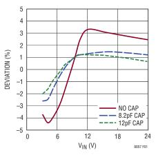
Figure 1. V<sub>OUT</sub> Line Regulation vs V<sub>IN</sub>
