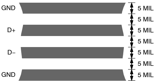
Figure 21. Typical Arrangement of Signal Tracks
