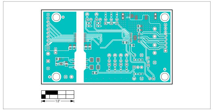
MAX14919 EV Kit PCB Layout — Top View
