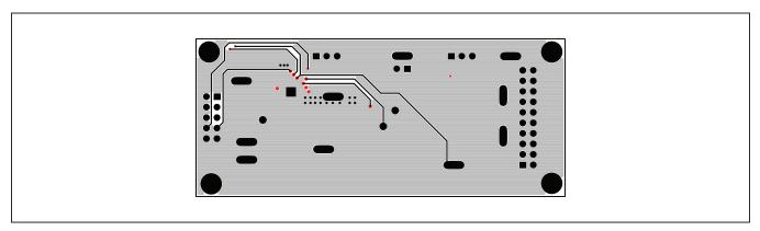
Figure 5. MAX20010 EV Kit PCB Layout—Layer 3
