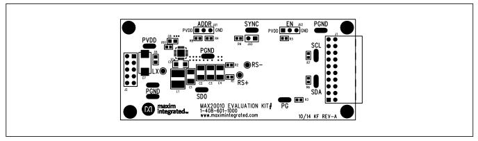
Figure 2. MAX20010 EV Kit Component Placement Guide—Component Side
