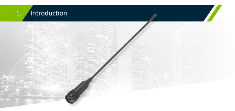
The FW.24 is a flexible 2.4GHz omni-directional whip antenna with an N type (M) connector for outdoor use. It features excellent efficiency (>75%) and high peak gain (>4 dBi) between 2400-2500MHz on a 30x30 cm ground plane.
