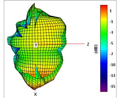
**Figure 11.** Radiation pattern XY plane, Figure 1 as reference (dB).
