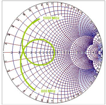
Figure 5. Smith Chart for the FXP290 Antenna.
