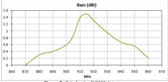
Figure 7. Gain for the FXP290 Antenna.
