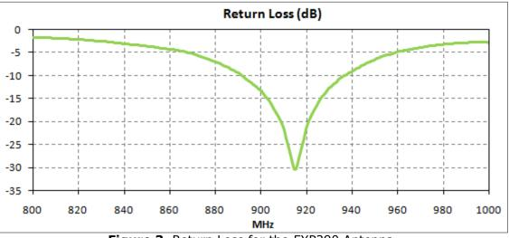
Figure 3. Return Loss for the FXP290 Antenna.
