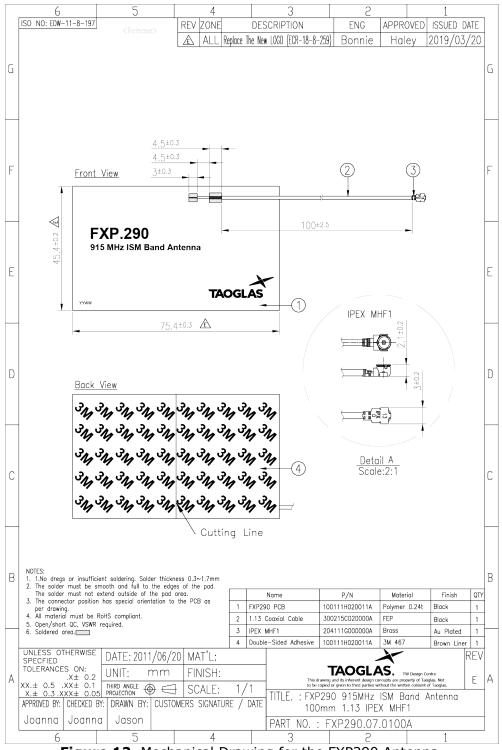
Figure 12. Mechanical Drawing for the FXP290 Antenna.
