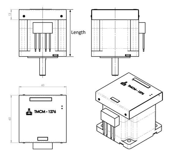
Figure 6: PD57/60-1276 all dimensions in mm
