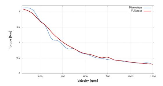
*Figure 9: PD60-3-1276 torque vs. velocity 24V / 2.8A, 256µsteps*
