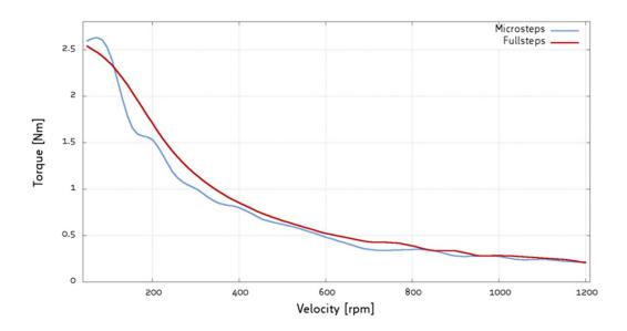
*Figure 10: PD60-4-1276 torque vs. velocity 24V / 2.8A, 256µsteps*
