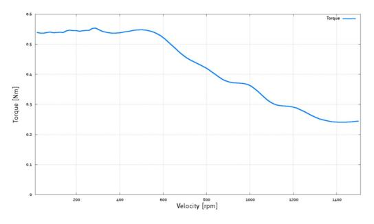
Figure 7: PD57-1-1276 torque vs. velocity 24V / 2.8A, 256 $\mu$ steps
