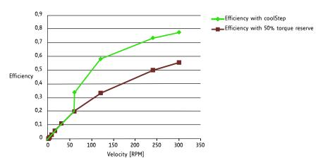
Figure 4: Energy Efficiency Example with coolStep
