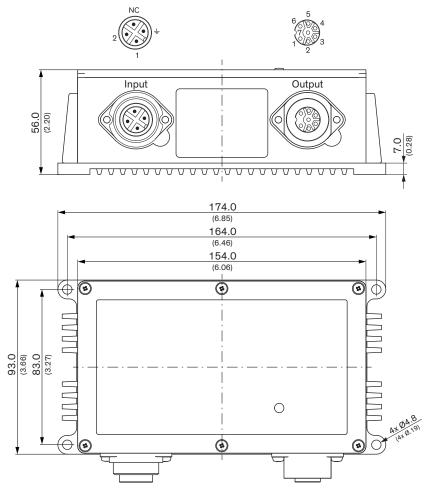
Pinout NC  $(\bullet)$ Output Input (male) (female) 1 1-3 L \_ 2 4-6 Ν + Ŧ ΡE 7 case
